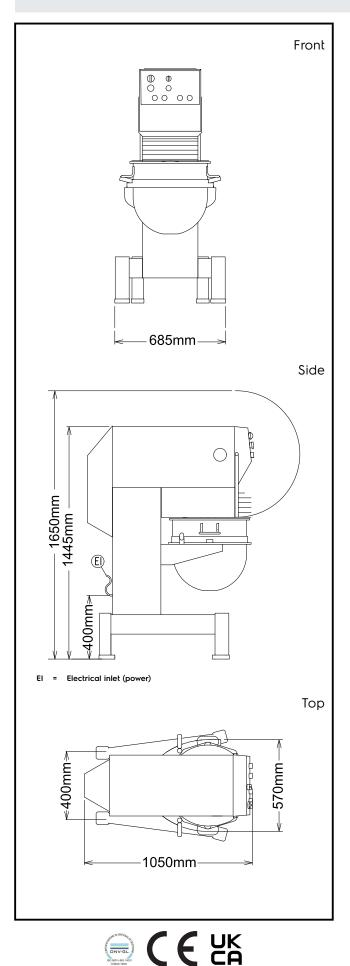
**Electric** Supply voltage: 380-440 V/3N ph/50/60 Hz Capacity: Performance (up to): 20 kg/Cycle Capacity: 60 litres
